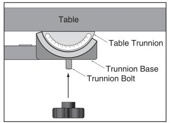
Figure 15. Installing the table onto the trunnion base.
